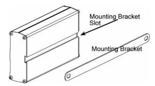
4. Attach the MultiModem with two screws to the mounting surface at the desired location on the equipment.
